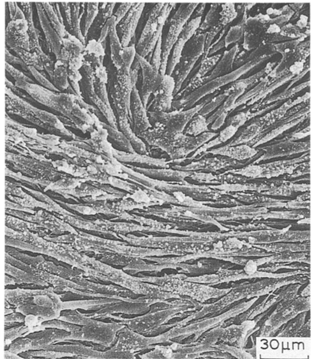
Figure 6 SEM micrograph of osteosarcoma cells cultured on poly lactide film (molecular weight 250 000)
